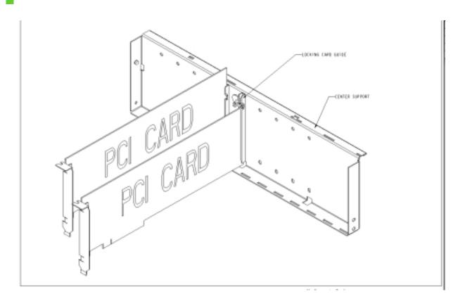
Figure 3-10: PCI Card Retention Mechanism
